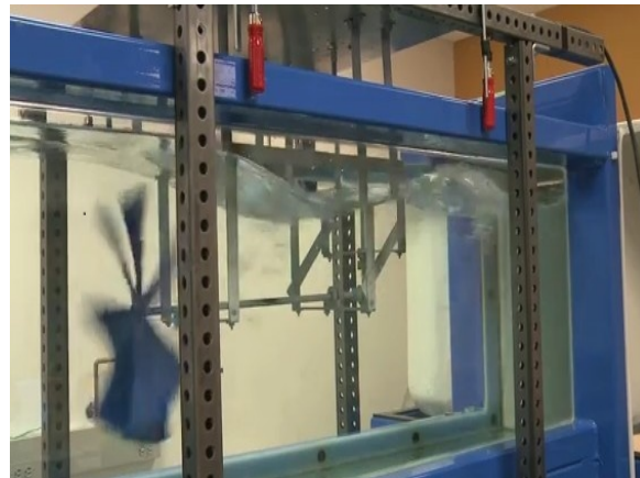
Fig. 10 A horizontal-axis hydrokinetic turbine with three blades under testing
