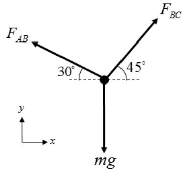
Determine the forces in the two rods in terms of  $m$ .
