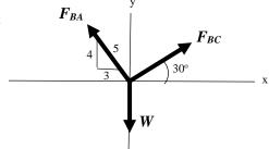
**Sum the forces:** The forces  $F_{BA}$  and  $F_{BC}$  can be found by summing the forces in the x and y directions.
