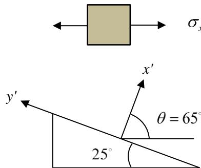
$$\sigma_x = \frac{F}{A} = \frac{F}{0.02(0.05)} = 1 \times 10^3 F, \quad \sigma_y = 0, \quad \tau_{xy} = 0, \quad \theta = 65^\circ$$
