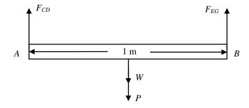
$$\begin{split} & \left( \sum_{A} + \sum_{A} M_{A} = 0 \right), \quad F_{EG}(1) - P(0.5) - W(0.5) = 0 \,, \quad F_{EG} = 0.5(W + P) \\ & \left( \sum_{A} + \sum_{A} M_{B} = 0 \right), \quad -F_{CD}(1) + P(0.5) + W(0.5) = 0 \,, \quad F_{CD} = 0.5(W + P) \end{split}$$
