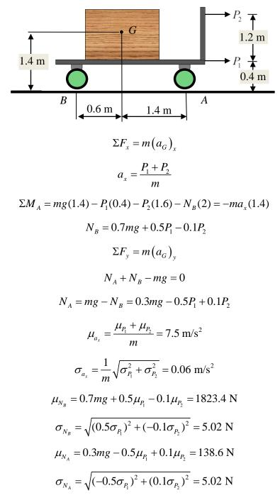
Therefore,  $a_x \sim N(7.5, 0.06^2) \text{ m/s}^2$ ,  $N_B \sim N\left(1823.4, 5.02^2\right) \text{ N}$ ,  $N_A \sim N\left(138.6, 5.02^2\right) \text{ N}$ . **Ans.**
