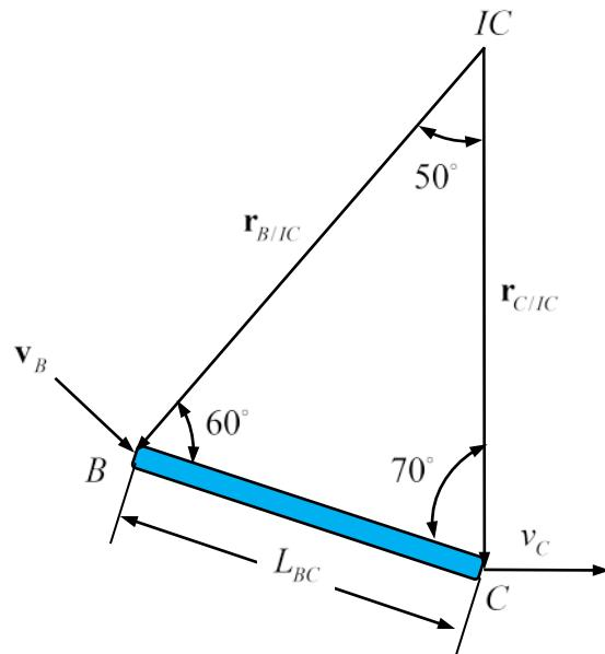
With the instantaneous center of zero velocity for BC as shown above, we have
