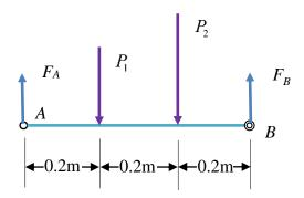
According to the moment equilibrium of rod AB with respect to point A,
